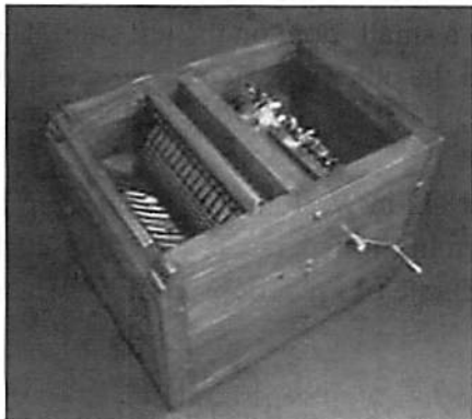
Photos: The 40-inch Reproduction of Eli Whitney's Cotton Gin: Model from The Smithsonian Institution, Washington, DC. Right:
