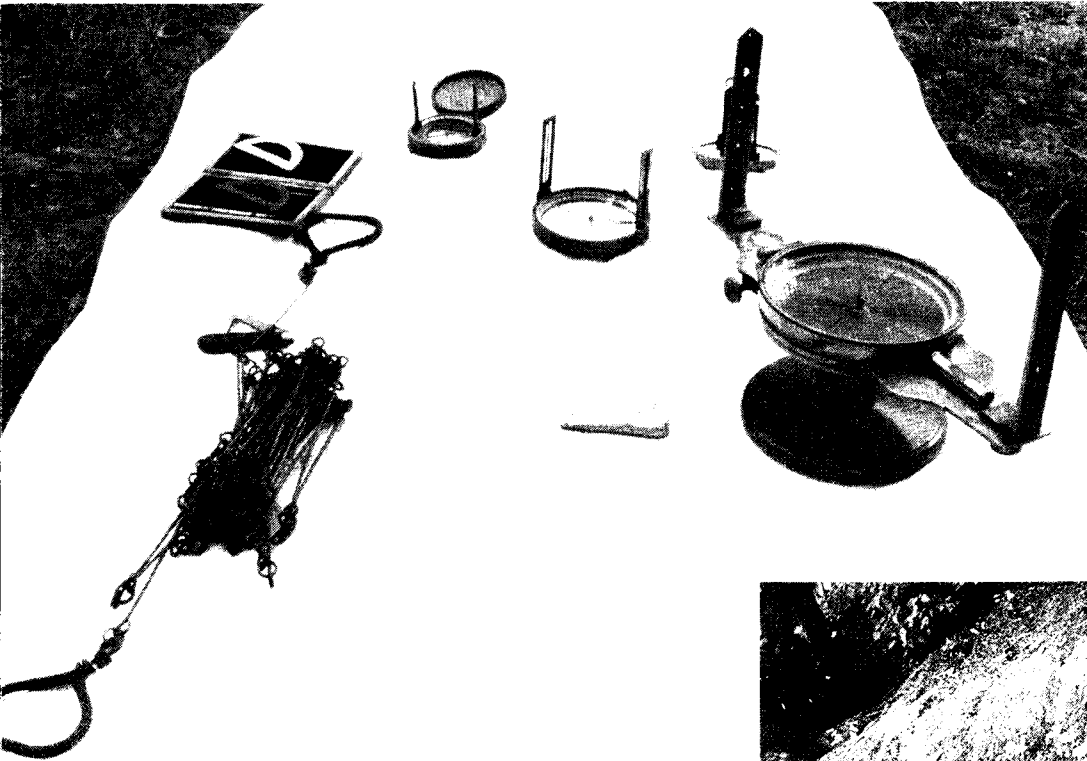
Early surveyors used chains and compasses to chart the mountainous border between North Carolina and South Carolina and recorded their work on a detailed 23-foot-long map. The second of two benchmarks established between 1811 and 1815, Commissioner's Rock cools its feet in the Chattooga River precisely on the 35th parallel.
